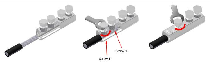
Stripping cable , see the stripping length  $(L_1)$  above a table. Before the installation, brush the contact surfaces with a wire brush and lubricate lightly with grease.
